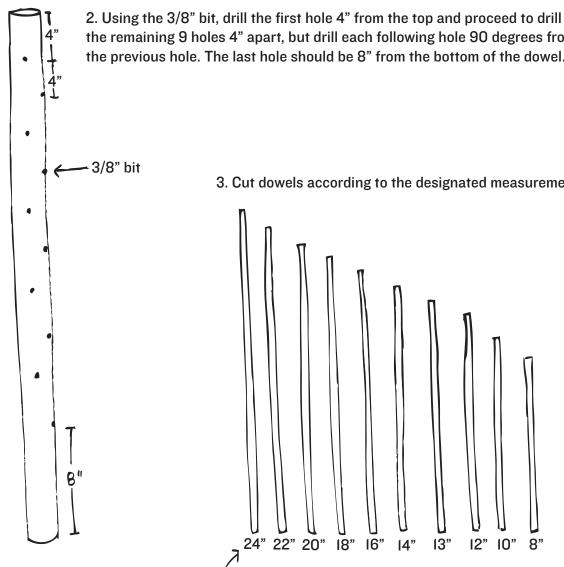
the remaining 9 holes 4" apart, but drill each following hole 90 degrees from the previous hole. The last hole should be 8" from the bottom of the dowel.
