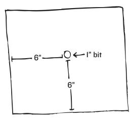
I. Using a I" bit, drill a hole in the center of the wooden base.
